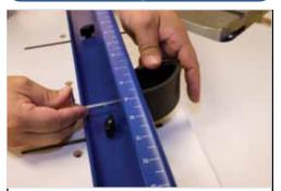
Mount the back locking jaw with two socket head bolts, washers and hex key wrench
