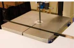
Adjust the plungers on the miter bar so the miter bar fits snug in the bandsaw miter slot.
