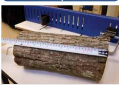
NOTE: Before making a cut, remove all the bark from the log if possible. Dirt and debris from the bark will dull and damage the bandsaw blade.
