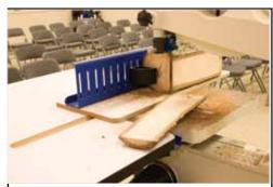
Now, rotate the log so the side you just cut is flat against the platform. Secure the log into the log mill and make your next cut. NOTE: You may have to make a series of cuts to reach your desired size and look. Step 7
