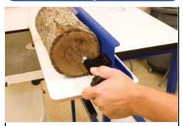
Adjust the back locking jaw to the appropriate mark on the scale.
