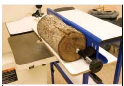
Using the platform as a guide, adjust the log and fence to maximize the yield of the log.
