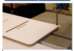
Locate the hole that is closest miter slot in relation to the bandsaw blade.
