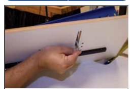
Place the log mill platform on top of the miter bar and align with the appropriate holes. Once aligned - secure the platform to the miter bar with the three machine screws. NOTE: If there is not enough room between the blade and the platform, you may have to cut the platform for proper use.
